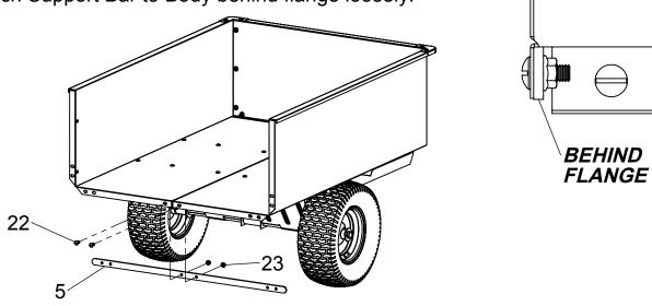
Assembly Instructions Attach Corner Gussets to Body and tighten all hardware. 6 22 Attach Tailgate to Body as shown. Tailgate must slide freely.
