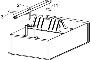
Slide Axle completely through Undercarriage; Drawbar and Spacer must be captured by Axle. Align Drawbar with Front Support and press down to latch.
