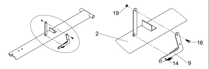
Attach hitch coupler plate to drawbar and tighten with hardware as shown.
