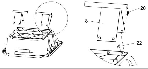
6 Attach front support loosely to poly body with hardware as shown.
