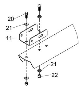
Attach 1-7/8" ball coupler to hitch plate on both sides and tighten with hardware as shown.
