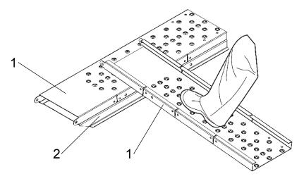
While standing or kneeling, place one foot or knee in center of upside-down ramp top and apply enough pressure to create bow as shown.
