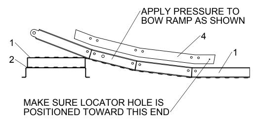
While applying pressure to ramp creating bow, add stiffener bar **INSIDE** ramp top flange as shown.
