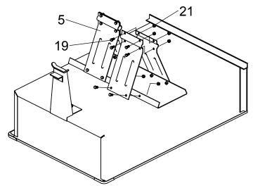
Attach latch and hitch bracket to drawbar with hardware as shown. Secure latch spring between latch and drawbar post.
