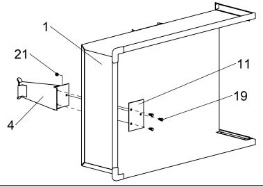
2 Attach axle holder plates to body loosely with hardware as shown.
