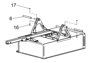
Slide washers and wheels onto stub axles as shown and install cotter pins. Bend legs of cotter pin to secure.
