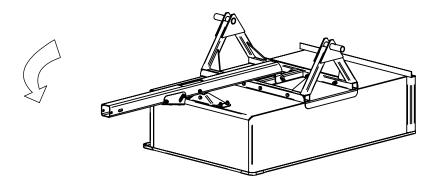
5 Insert stub axles into undercarriage and secure with pins as shown.
