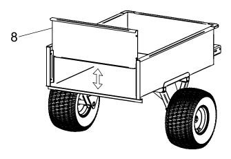
8 Attach ball hitch to drawbar with spacers and hardware as shown.
