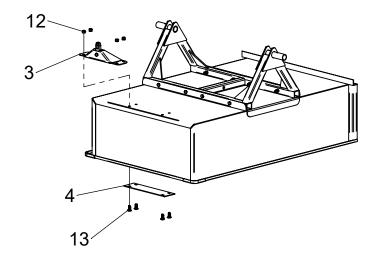
Align holes in swivel clevis and undercarriage and install pin as shown. Secure pin on both ends with hairpins.
