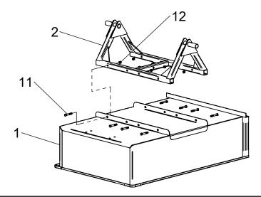
2 Attach front support to body securely with hardware as shown.
