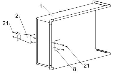
2 Attach axle holder plates to body loosely with hardware as shown.
