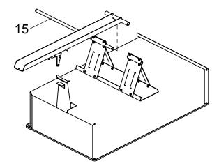
Slide axle completely through undercarriage; be sure to catch the drawbar when sliding the axle. Align drawbar with the front support and press down firmly to latch.
