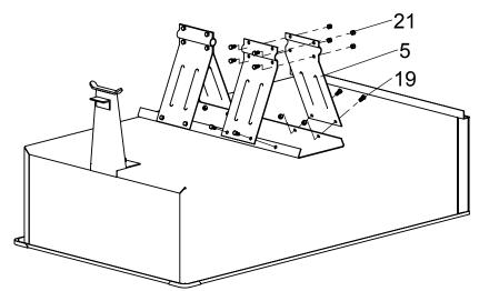
Attach latch and hitch bracket to drawbar with hardware as shown. Secure latch spring between latch and drawbar post.
