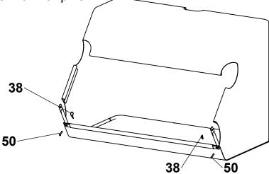
9 Insert Top Frame Tubes into Rear Frame Tube and snap into position.
