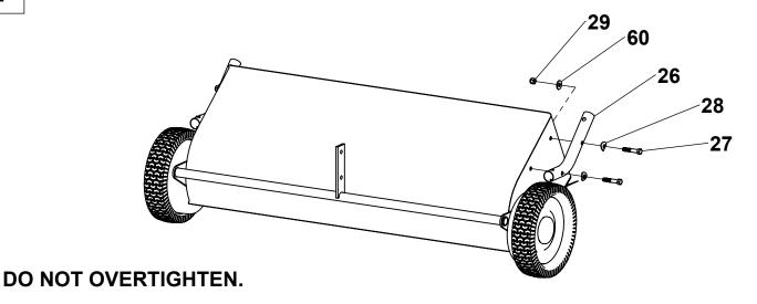
2 Attach Handle to Height Adjustment and tighten hardware.
