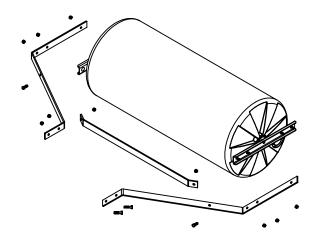
Attach the rear bar to the side channels and loosely tighten hardware. Add clevis bars on top and bottom of the side bars and loosely tighten. Complete assembly by tightening all hardware.
