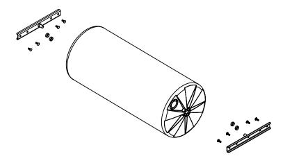
Attach the side bars onto the side channels and loosely tighten hardware as shown. Place support bar in between the side bars and loosely tighten all hardware.
