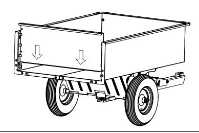
12 Install hitch pin and hairpin to secure to attachment vehicle.
