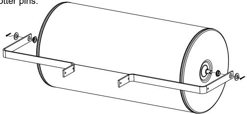
Add roller hitch weldment to side bars using 3/8" bolts and 3/8" nuts.
