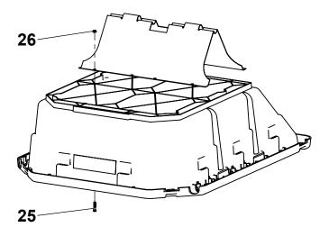
2 Attach Front Support to Poly Body and tighten hardware.
