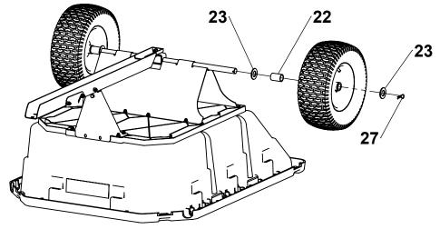
6 Install Hitch Pin as shown.
