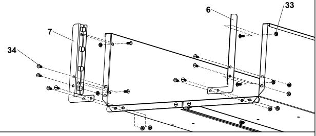
11 Attach tailgate to body as shown. No hardware required, tailgate should move freely up or down.
