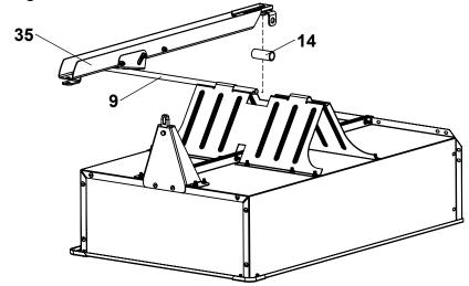
Slide axle completely through undercarriage; be sure to catch the drawbar when sliding the axle. Align drawbar with the front support and press down to latch.
