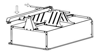
8 Slide washers, spacers, and wheels onto axle and secure with hairpins as shown.
