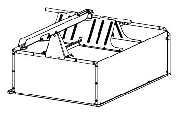
Slide Washers, Spacers and Wheels onto Axle and secure with Hairpins as shown.
