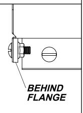
Attach Corner Gussets to Body and tighten all hardware.
