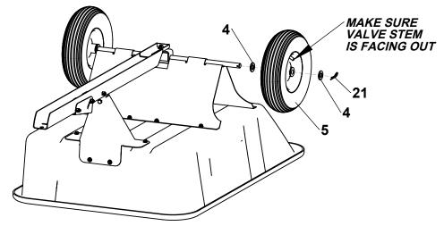
6 Install spring loaded hitch pin as shown.
