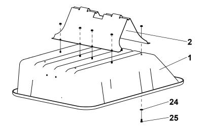
2 Attach Front Support loosely to Poly Body as shown.
