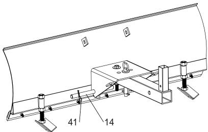
Slide hanger bolt through bottom hook of spring. Attach top hook of spring to top bracket on the snowplow. Insert hanger bolt through tab on the pivot plate and tighten 3/8-16 nyloc until spring begins to expand.
