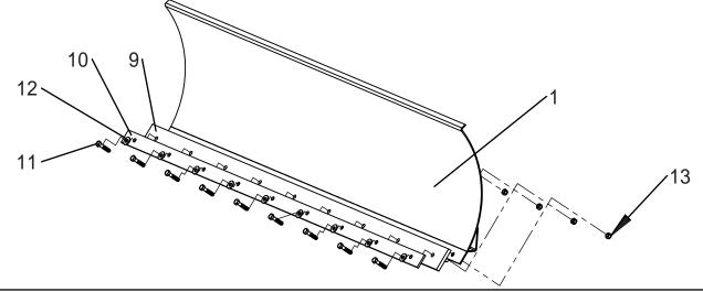
6 Install Skid Shoe assembly with 3/4-10 hex nuts. Tighten nuts into tube to set the desired height of blade off the ground.
