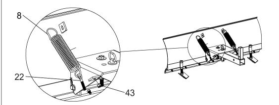
NOTE: ONLY TIGHTEN NUTS UNITL SPRING COILS BEGIN TO SEPERATE.
