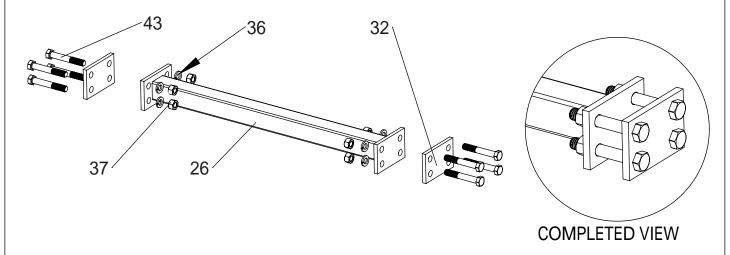
Slide previous assembly over foot lift tube and tighten bolts. Insert foot pedal assembly into clamping bracket and tighten bolts. Adjust each clamping feature so the blade can be raised to the desired height.
