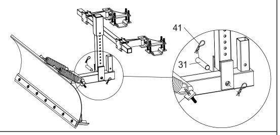
1 1 Attach foot lift tube to lower frame assembly with 3/8" x 1-1/4" pin and secure with hairpin cotter.
