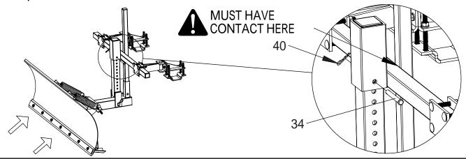
13 Attach foot lift assembly to lock plates using 3/8-16 x 2-1/2 bolts, 3/8" lock washers and 3/8" hex nuts. Loosely attach bolts and lock plates.
