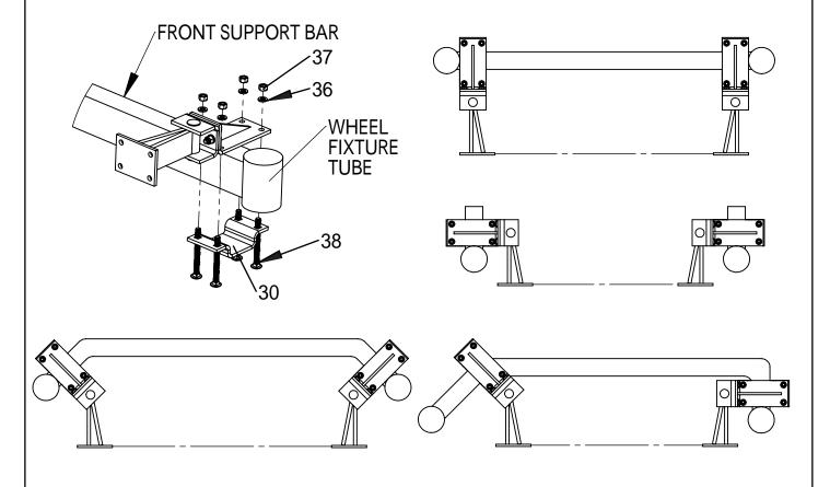
Install mounting bracket plate with 3/8-16 x 2-3/4" carriage bolts, 3/8" lockwashers and 3/8-16 hex nuts. Loosely attach bottom bolts first and slide horizontal mounting bar from above. Center the horizontal tube on the mower and slide vertical adjustment tube into tube from below. Add top row of bolts and tighten bolts and nuts.
