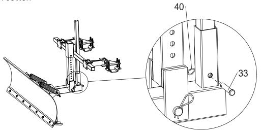
Push Snow Blade towards tractor until there is contact between the foot lift tube and horizontal mounting bar. Once in position, insert 3/8" x 2-3/4" pin through horizontal mounting assembly and vertical rotation assembly. Secure with hairpin cotter.
