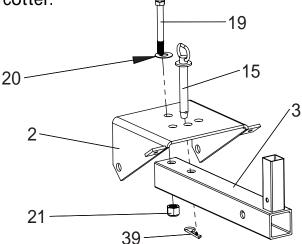
Slide blade pivot rod through lower holes in pivot plate and brackets on the snowblade. Secure on both sides with hairpin cotters.
