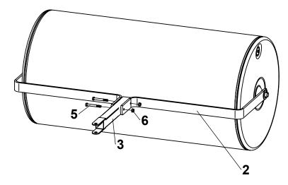
Add Hitch Pin (9) into clevis of Hitch Weldment (3) and secure with Hairpin Cotter (10).
