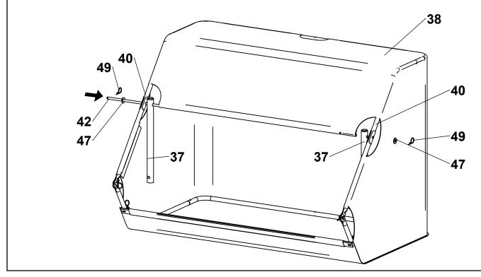
Unscrew Thumb Screw from Tension Tube Assembly (44). Next, Hold Hopper Bag (38) open and carefully insert Tension Tube Assembly (44) through opening in Hopper Bag and into hole in bottom Center Frame Tube (41). Pull top Center Frame Tube over tension tube and align holes. **OPENING** 42~ 38 SHOWN INSTALLED
