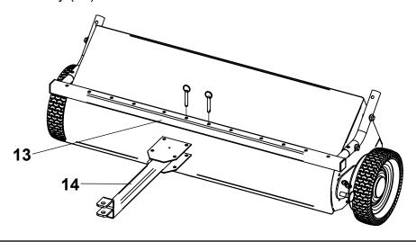
First remove factory hand tightened nuts from studs. Use nuts to attach Height Adjustment Handle (15) Using a 9/16" Open End Box Wrench.
