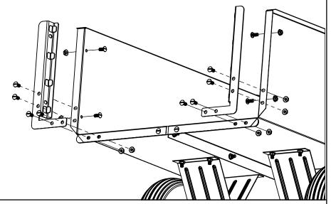
1 1 Attach tailgate to body as shown. No hardware is required, tailgate should move freely up or down.
