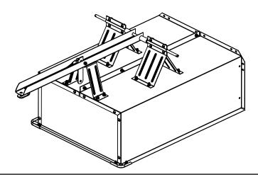
Slide washers and wheels onto axle and secure with hairpins as shown.
