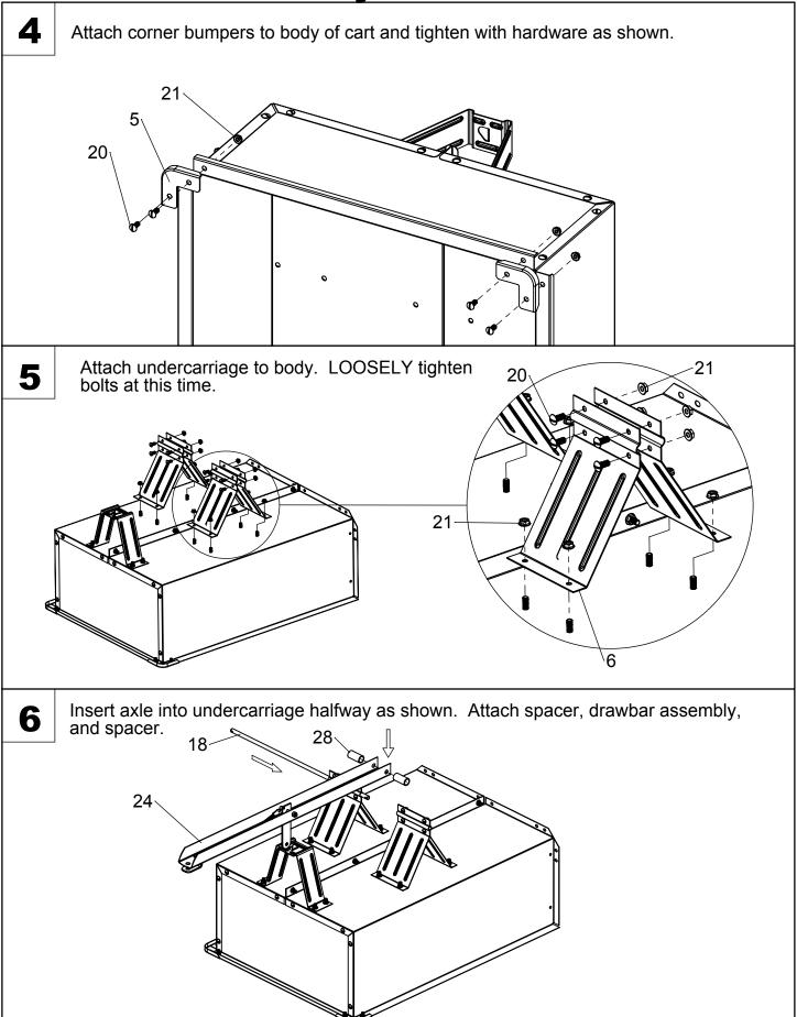
Slide axle completely through undercarriage; be sure to catch the drawbar when sliding the axle. Align drawbar with the front support and press down to latch.
