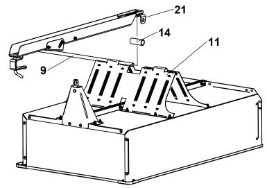
Slide Axle (9) completely through Undercarriage (11); be sure to catch the Swivel Clevis (21) and Spacer (14) when sliding the Axle (9) through. Align drawbar with the Front Support (16) and press down to latch.
