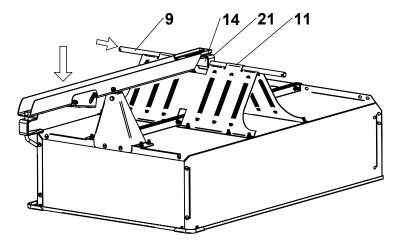
Slide Washers (12), Spacers (13), and Wheels (10) onto Axle (9) and secure with Hairpins (15) as shown.
