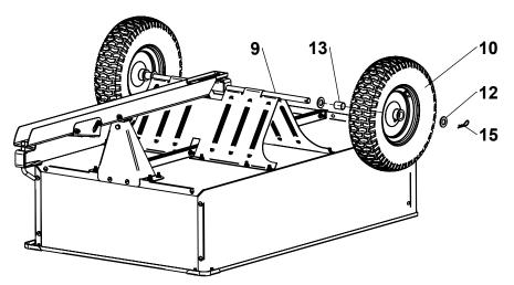
Attach the Support Bar (8) to body behind flange loosely as shown.
