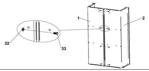
Attach Front Support (16) to Body Halves (1 & 2) and tighten hardware (32 & 33) as shown.
