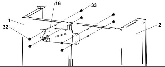
Attach Undercarriage (11) to Body Halves (1 & 2) and tighten hardware (32 & 33).
