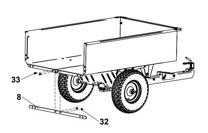
10 Attach Corner Gussets (6 &7) to rear and sides of body and tighten with hardware (32 & 33) as shown.
