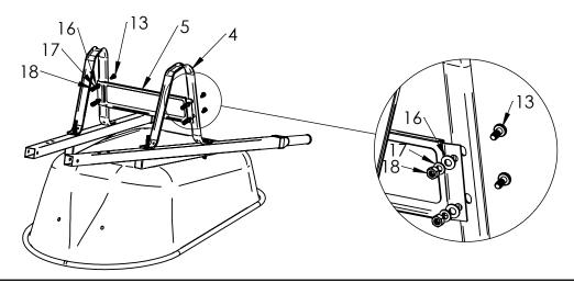
Install Dump Bracket (6) onto Handles (3) with 2-1/8" Bolts (14), Washer (16), Split Washer (17), and Hex Nut (18) hand tight. DO NOT tighten hardware until final step.
