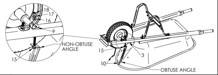
Insert 3/4" Bolt (13) through Body (1). Push Body Support (10) over Bolt (13). Secure by installing Washer (16), Split Washer (17), and Hex Nut (18) hand tight. All parts and hardware are now in place. Tighten all hardware in order of install.
