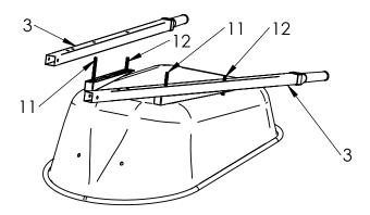
3 Slide Legs (4) over Bolts (11 & 12). Install Washer (16), Split Washer (17), and Hex Nut (18) hand tight. DO NOT tighten hardware until final step.
