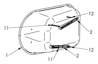
Assembly Tip: Temporarily secure bolt head to body with tape.
